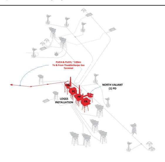
Figure 1.6.2: LOGGS Installation Layout
