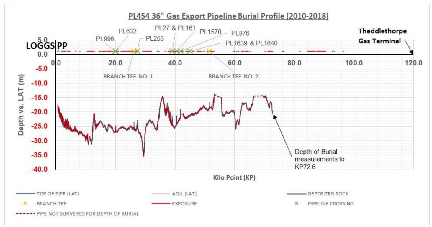
Figure A1.1.1: PL454 Seabed & Burial Profile (2010-2018)<sup>11</sup>
