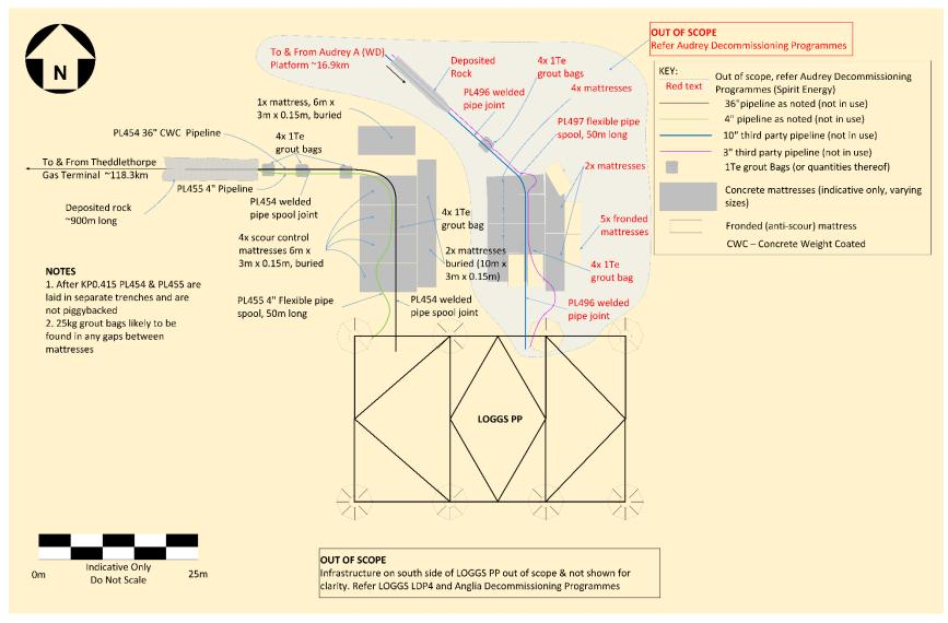
Figure 2.3.7: Approaches & Pipelines LOGGS PP North Side
