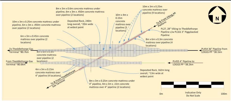
Figure 2.3.5: Pipeline Crossing PL454 & PL455 over PL27 & PL161
