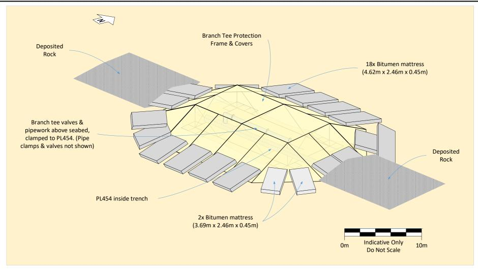
Figure 2.3.2: Schematic Branch Tee No. 1<sup>5</sup>
