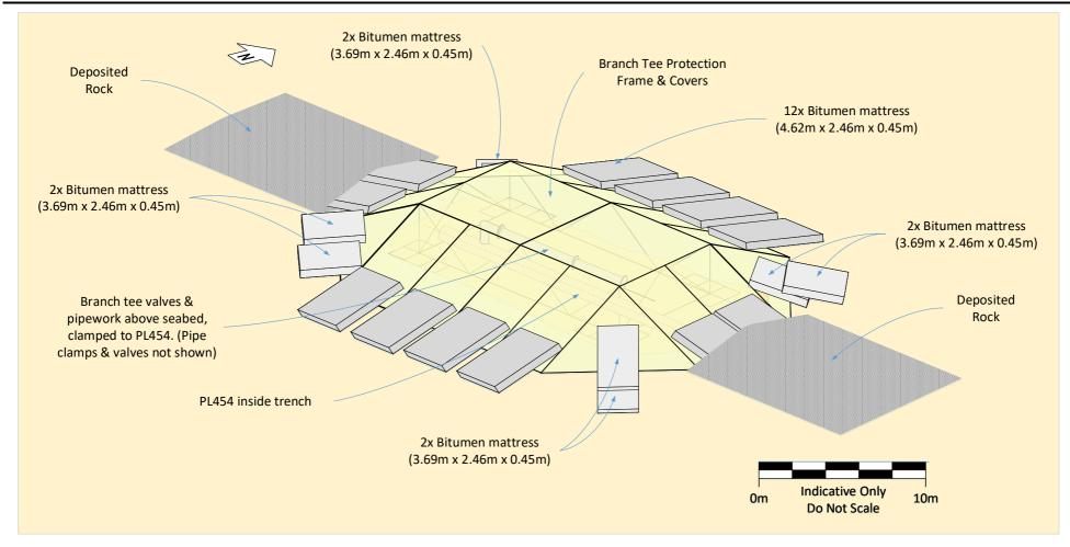
Figure 2.3.3: Schematic Branch Tee No. 2
