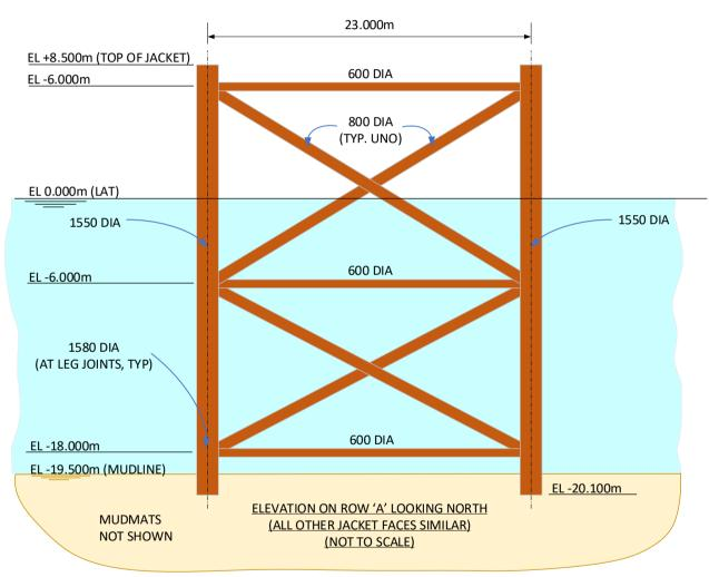
Figure 3.2.1: LOGGS PR Jacket Typical View
