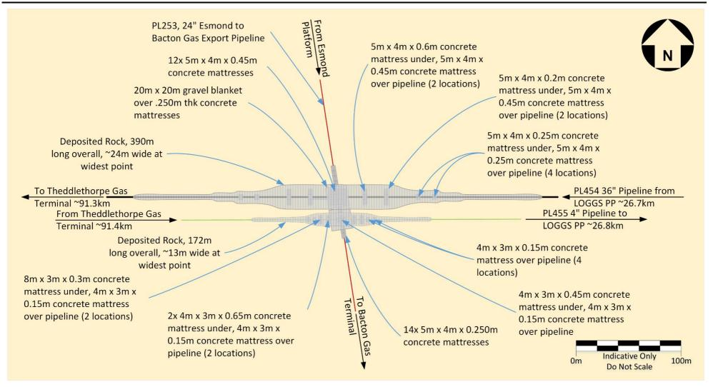
Figure 2.3.4: Pipeline Crossing PL454 & PL455 over PL253
